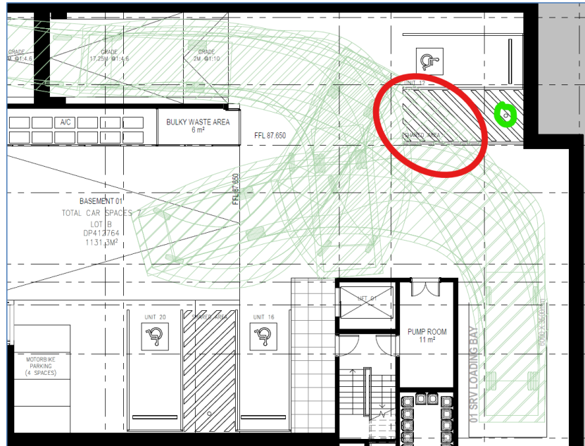
Figure 1: Conflict between accessible parking space and manoeuvring
